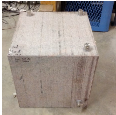
Figure 7: Sample G01-93 with sensors attached
